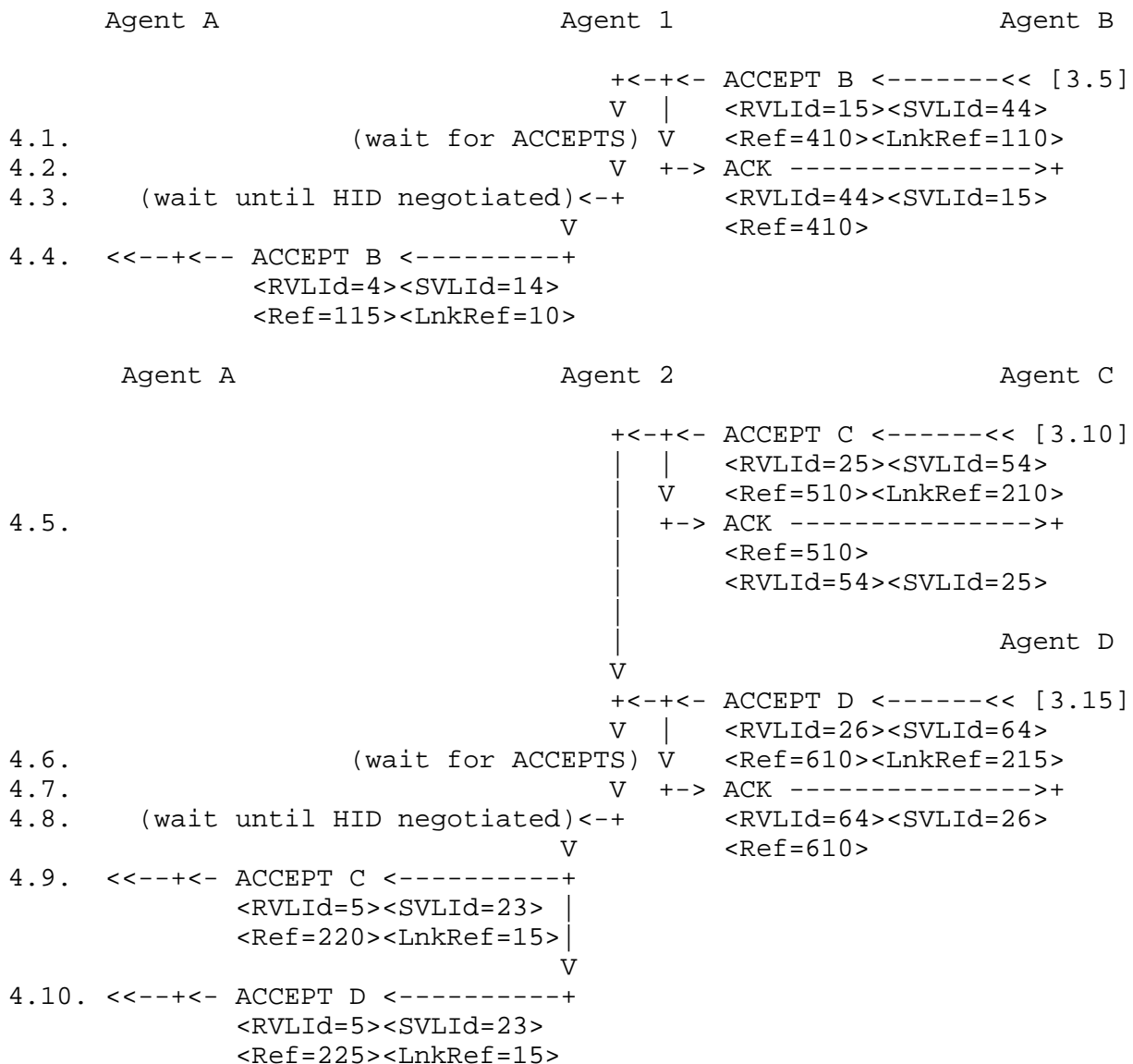
Figure 8. ACCEPT Processing by an Intermediate Agent
